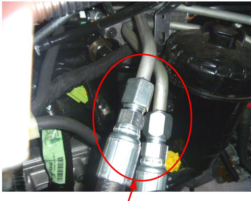
**Cut transmission cooler lines and install hoses using the compression fittings making sure to get them tight enough without collapsing tube to prevent leaking.**
