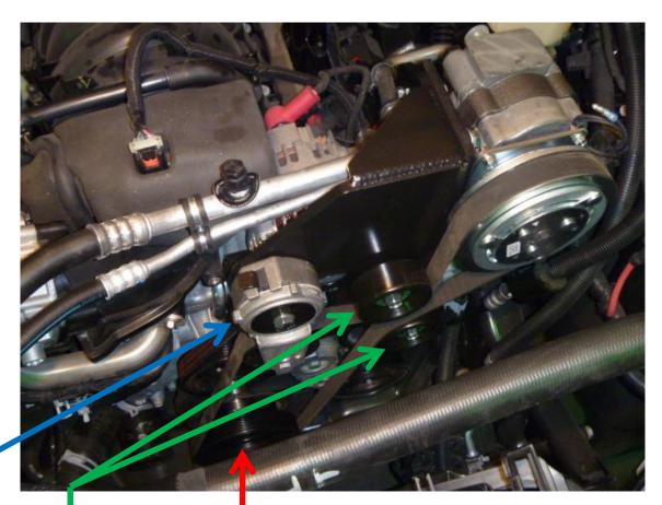
Remove harmonic balancer bolt. Install new drive pulley(1) using bolt(2) and flat washer(3). Before torquing the bolt, rotate the pulley counter clockwise until the drive studs make contact with the spokes in the balancer. Torque bolt(2) to 135 ft/lbs.
