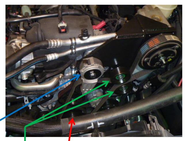
Remove harmonic balancer bolt. Install new drive pulley(1) using bolt(2) and flat washer(3). Torque bolt(2) to 135 ft/lbs.). Before torquing the bolt, rotate the pulley counter clockwise until the drive studs make contact with the spokes in the balancer.
