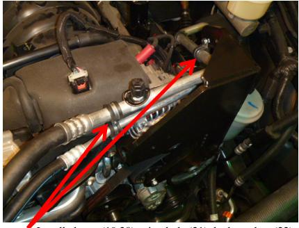
Install clamps(19,20) using bolts(21), lock washers(22) and nut(23).
