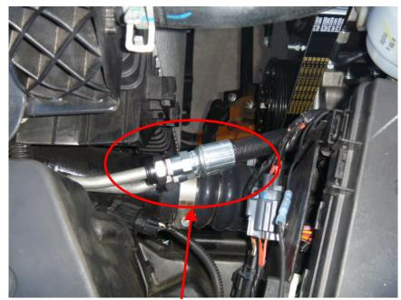
Install quick clip end of hoses to radiator side.
