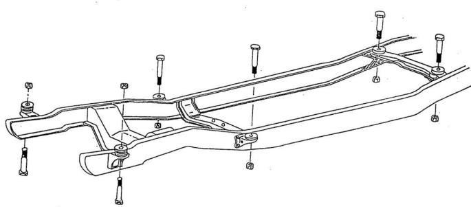
Moving cab forward requires loosening six body mount bolts. Two bolts by radiator are reached from under the truck, loosen until rubber bushings feel loose, do not remove bolts. Two bolts are under floor mat (one is under brake pedal) which require laying floor mat/carpet back to gain access to small covers which conceal bolts. Move seat ahead for access to rear bolts, loosen four cab bolts until finger loose, do not remove bolts.
