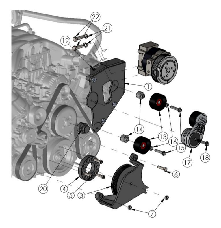
**EMK534-8SB-5.5** 2016-2019 Ford F650-750 6.8L V10 3 Valve W-WO AC W/Bearing Support
