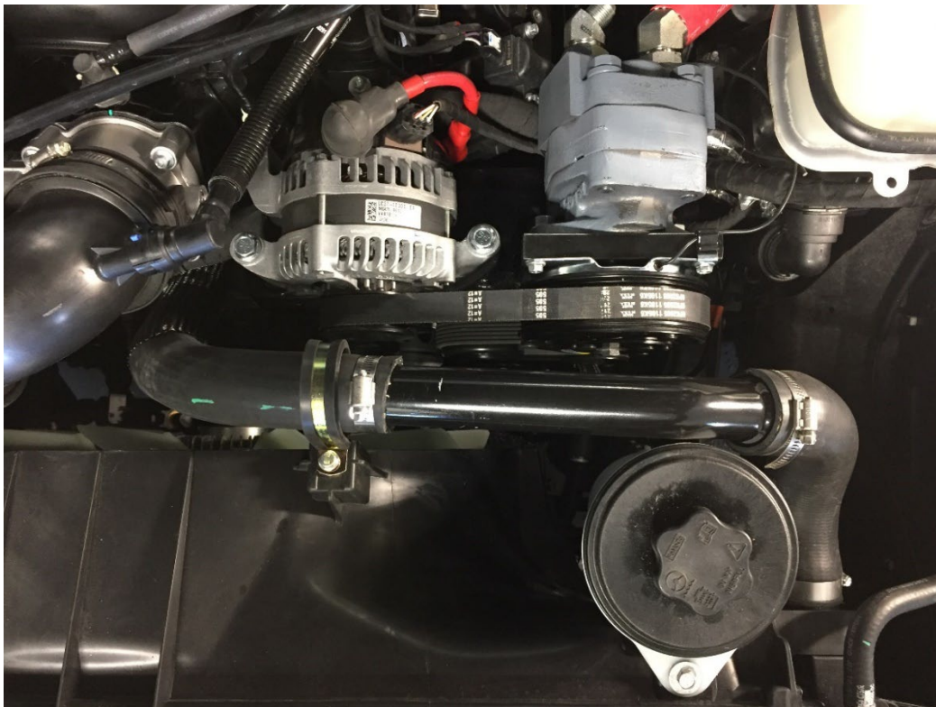
As Shown: Auxiliary Clutch Pump Application
