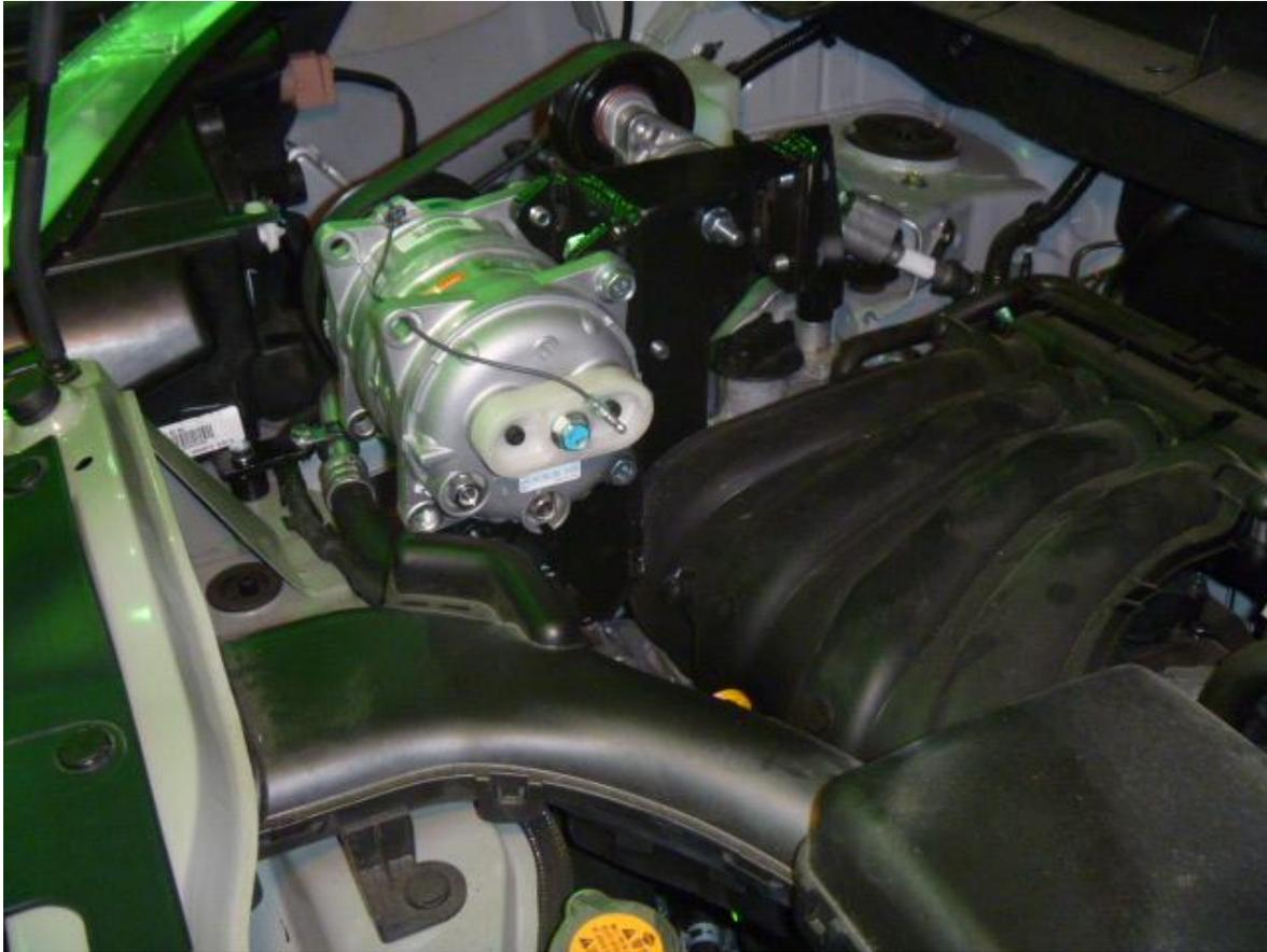
Secure the O.E.M. air conditioner line to upper radiator support with bracket (8) using bolts (9,18), lock washers (10,19), and wire loom clamp (17) as shown above.
