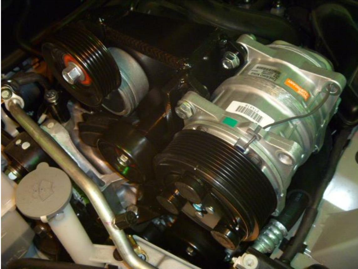
Install one of the flat idlers (13) with short bushing (14) and bolt (7) to lower mount on main bracket. Install the idler with shoulders on both sides (15) with long bushing (16) and bolt (4) to upper idler mount on main bracket. Install tensioner (11) to main bracket using nut (12). After moving the factory air conditioner line out of the way, install aux. air conditioner compressor using bolts (7,20), nuts (12) and slide bushings (21).
