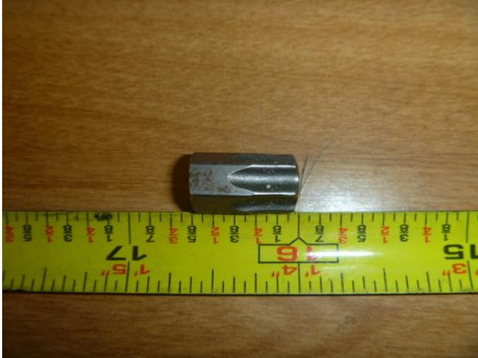
Use Gearwrench part number 85035 to remove tensioner by shortening the T50 driver bit to approximately 5/8" as shown above. It may be necessary to use a cheater pipe to get it loose. Don't unscrew the bolt enough to where the tool can't be removed. Use the tips of your fingers to unscrew the rest of the way.
