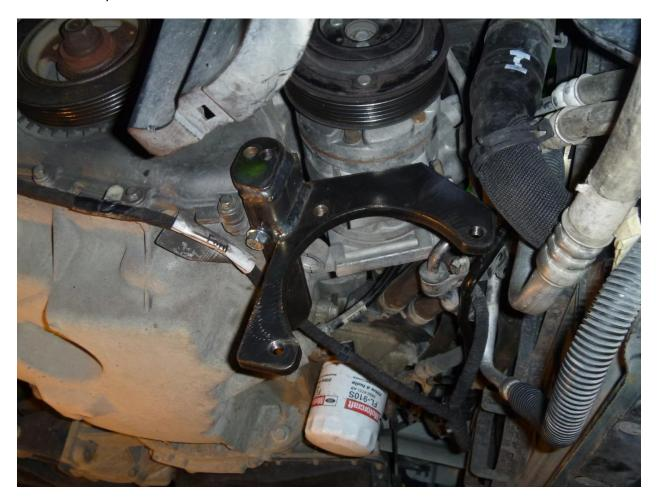
Remove the two front side bolts from oil pan on passenger side and discard.
