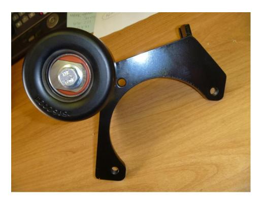
After belt is installed, loosen the idler bolt slightly and then rotate eccentric 180 deg. as shown above and retighten idler bolt. It may be necessary to actuate tensioner in this process. This is done in order to make belt installation easier and then gain additional belt take up that is needed.
