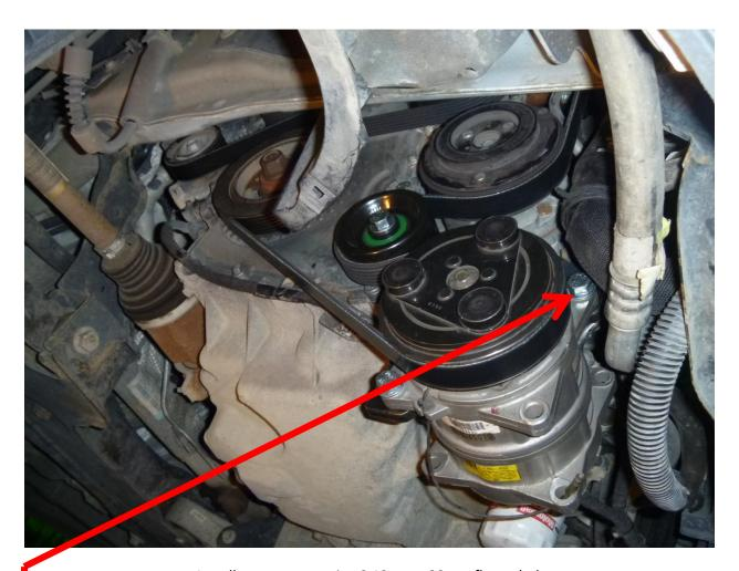
Install compressor using 3 10mm x 30mm flange bolts.
