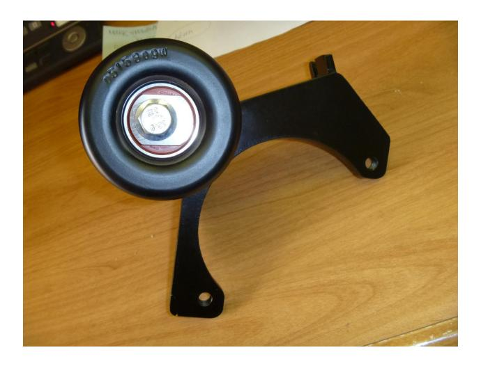
Install idler in this order 1-washer, 1-Gates 38005 idler, 1-piloted eccentric and then 1-10mm x 30mm flange bolt with eccentric rotated in position shown above. Idler should be installed in the hole to the left or closest to the crank pulley.
