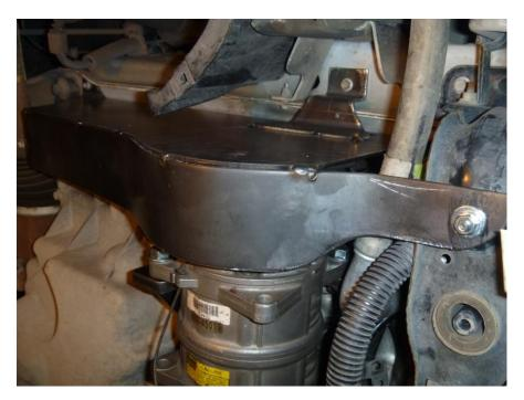
Install new splash shield reusing OEM bolts in frame and (1)  $1/4 \times 3/4$  bolt, (2) 1/4 flat washers, (1) 1/4 Lock washer and (1) nut in radiator supports as shown. Replace engine coolant.
