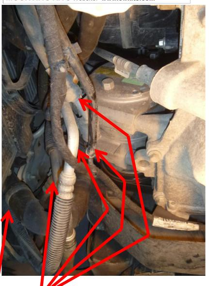
After draining coolant and removing lower section of lower radiator hose bend these four lines forward toward radiator to gain enough clearance for mounting bracket. Hose coming off of tee in lower radiator hose may need to be removed and replaced on other side of factory air conditioning hoses to prevent hose from rubbing on radiator shroud.
