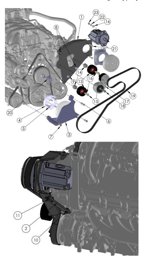
2017-2019 Ford F450-550 Cab Chassis 6.8L V10 Triton 3 Valve For use W-WO AC / Requires SAE Two Bolt "A" Flange Pump / Requires 8 Groove Clutch
