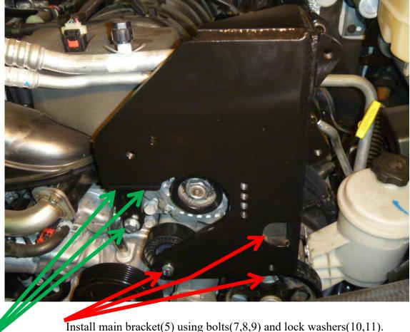
install main bracket(5) using bolts(7,6,5) and lock washers
