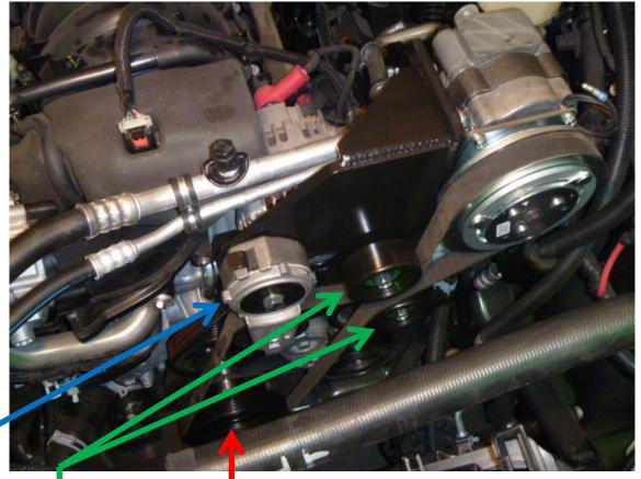
Remove harmonic balancer bolt. Install new drive pulley(1) using bolt(2) and flat washer(3). Before torquing the bolt, rotate the pulley counter clockwise until the drive studs make contact with the spokes in the balancer. Torque bolt(2) to 135 ft/lbs.
