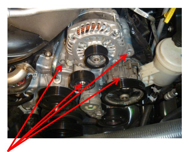
Remove the bolts from these locations. Remove the standoff for the air conditioner lines.
