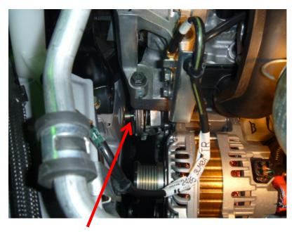
Once bolt is unscrewed, pull bolt head out to the frame of the van while pushing the tensioner up against its mounting location as shown above. Use a pneumatic reciprocating saw to cut the bolt as close to the tensioner as possible (it may be necessary to use a carbide edged reciprocating or sawzall blade). Once this is done, the tensioner should be able to be removed.
