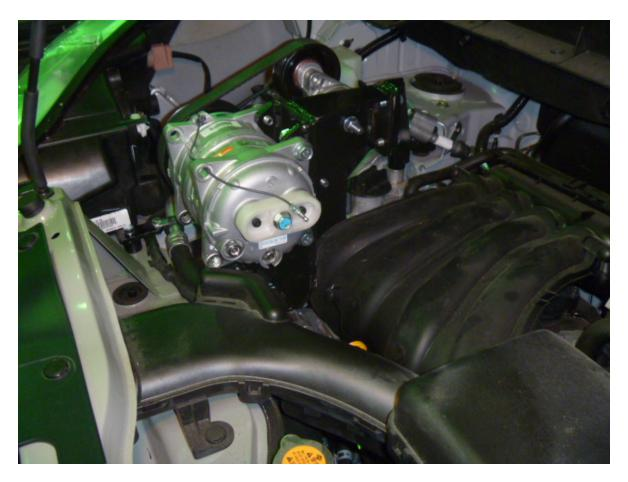
Secure the O.E.M. air conditioner line to upper radiator support with bracket (8) using bolts (9,18), lock washers (10,19), and wire loom clamp (17) as shown above.
