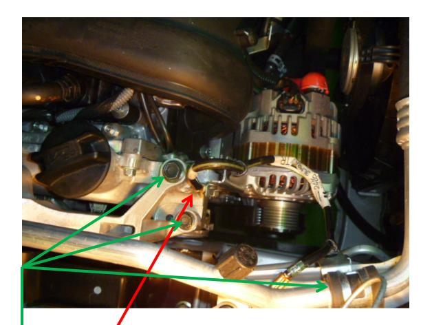
Remove this end of ground cable and remove from clamps. Loosen opposite end of cable so that the ground cable can be installed on the upper left hand side of the timing cover. Remove that timing cover bolt and install the ground clamp reusing the bolt. Tighten both ground clamp bolts.
