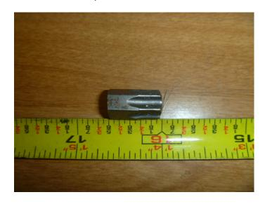
Use Gearwrench part number 85035 to remove tensioner by shortening the T50 driver bit to approximately 5/8" as shown above. It may be necessary to use a cheater pipe to get it loose. Don't unscrew the bolt enough to where the tool can't be removed. Use the tips of your fingers to unscrew the rest of the way.
