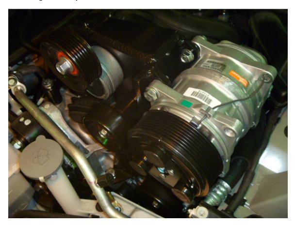
Install one of the flat idlers (13) with short bushing (14) and bolt (7) to lower mount on main bracket. Install the idler with shoulders on both sides (15) with long bushing (16) and bolt (4) to upper idler mount on main bracket. Install tensioner (11) to main bracket using nut (12). After moving the factory air conditioner line out of the way, install aux. air conditioner compressor using bolts (7,20), nuts (12) and slide bushings (21).
