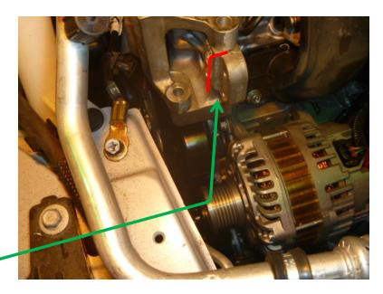
Cut off this boss approximately along the line shown using a sawzall or other suitable tool. Cover the alternator with a rag before cutting to keep shavings out of the alternator.
