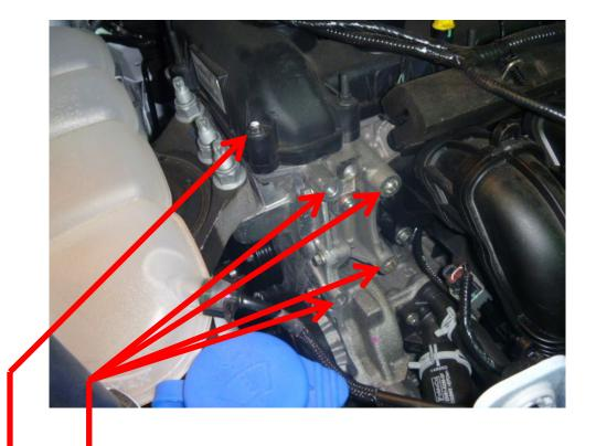
Install the main bracket(1) using the bolts(2) in the rear holes and Bolts(3) in the front holes.
