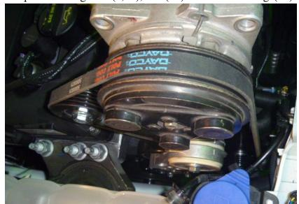
Install the belt(19) according to the diagram below. Belt must be slipped under the tensioner idler, then the tensioner bolt tightend. Belt should be installed in center 4 grooves on the compressor.
