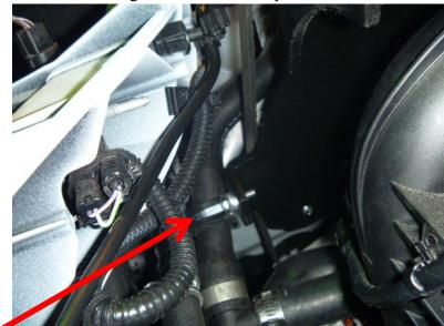
Secure the coolant line using clamp(12), bolt(14) and lock washer(13).
