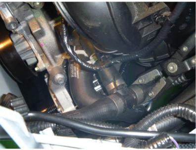
Cut the band off of the coolant line shown above. Using hose pinching pliers on the left and right side of the "T", remove the section of hose that the band was cut off of and replace with the new section of hose(10) using clamps(11).
