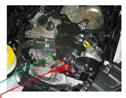
Install the main bracket(1) re-using the O.E.M. bolts. Finger tighten bolts.
