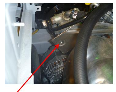
Remove the bolt from the power steering pump at this location.
