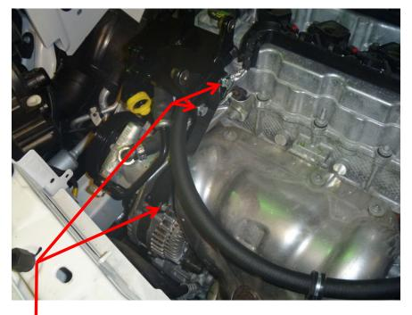
Install brace(2) using bolts(6,8) and lock washer(7).
