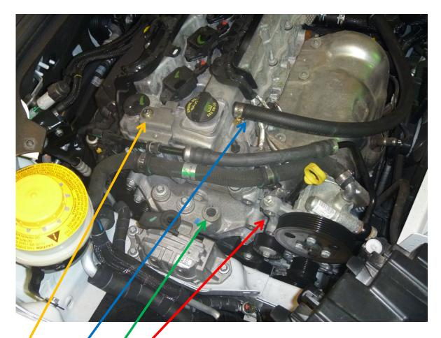
Remove the front power steering brace from this location.
