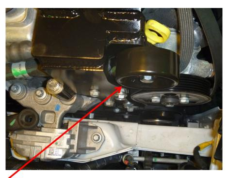
Install idler(10) using bushing(9) and bolt(11).
