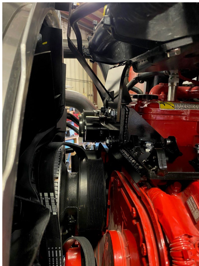
Fan Ring Support Bracket Installed
