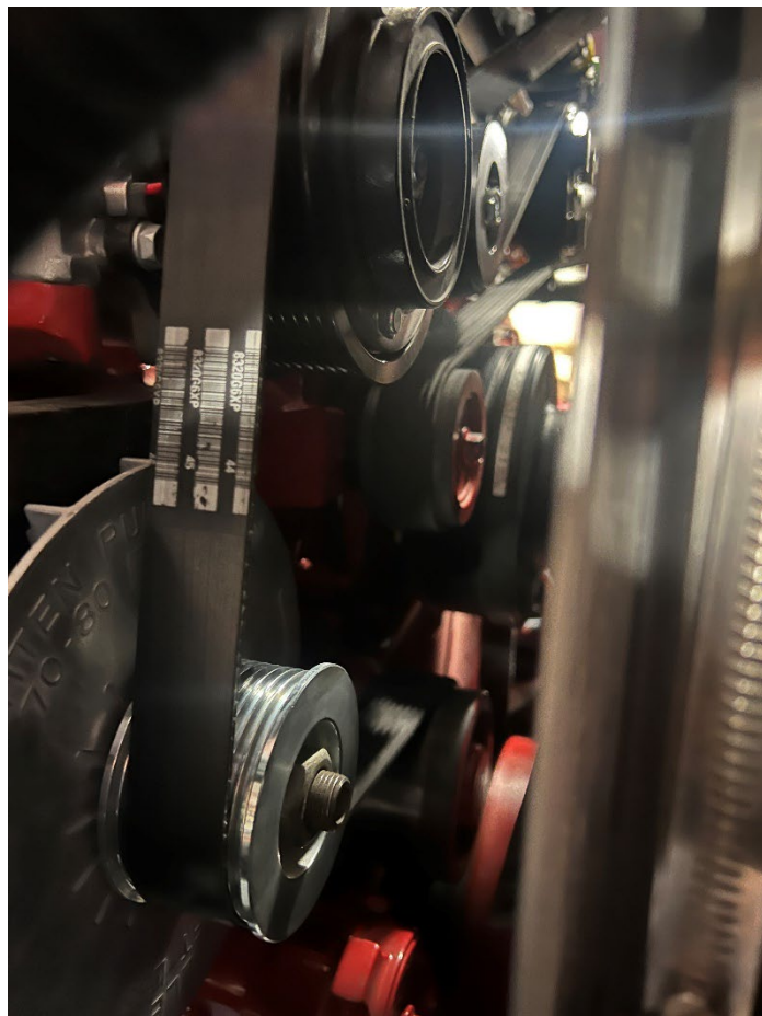
Idler Mounting Bracket Installed
