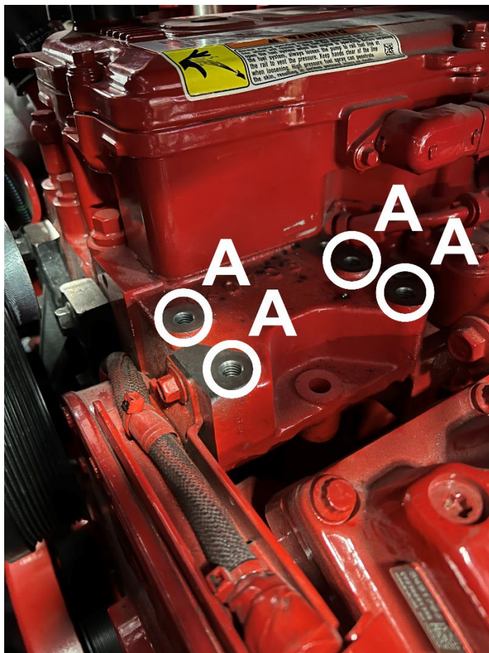
Main Bracket Mounting Locations [A]
