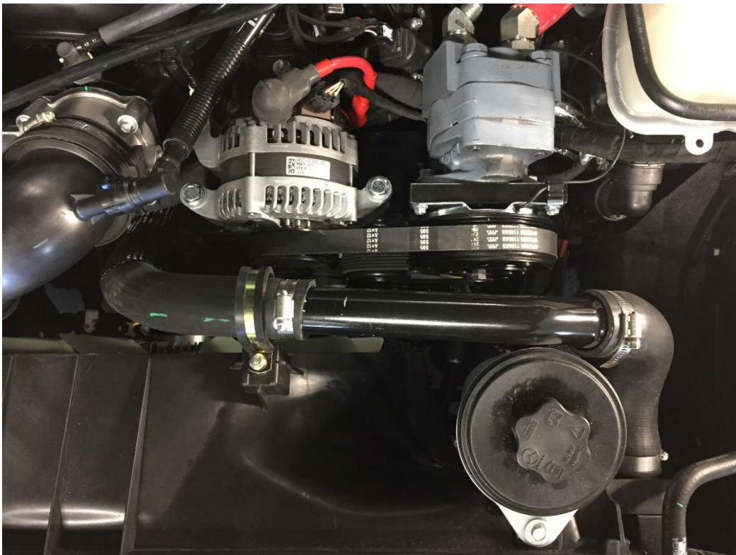
As Shown: Auxiliary Clutch Pump Application
