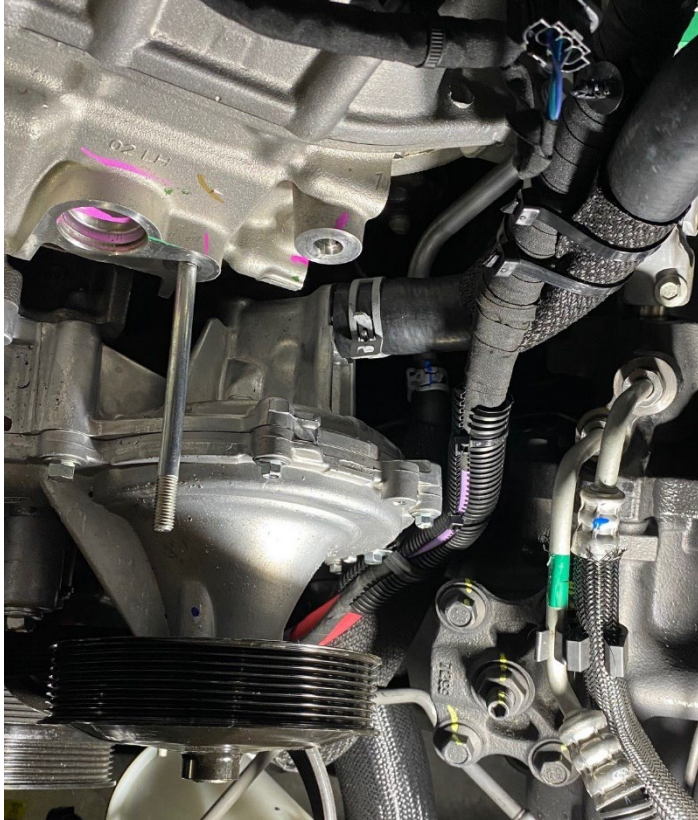
Battery Cable Support Hardware (18-22)
