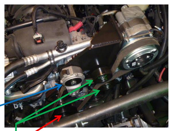
Remove harmonic balancer bolt. Install new drive pulley(1) using bolt(2) and flat washer(3). Before torquing the bolt, rotate the pulley counter clockwise until the drive studs make contact with the spokes in the balancer. Torque bolt(2) to 135 ft/lbs. Install the three 8mm set screws(26) into the drive pulley from the inside. Run them all out until they touch the damper evenly. Then, tighten each set a little at a time until you reach 15-20 inch pounds.
