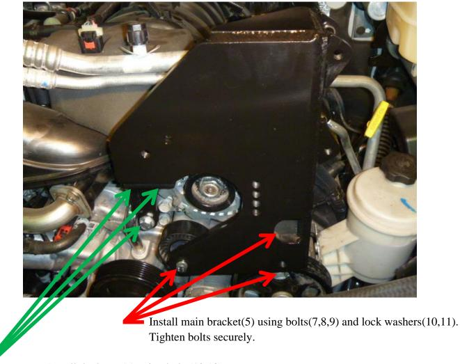
Install the brace(6) using bolts(12,13).
