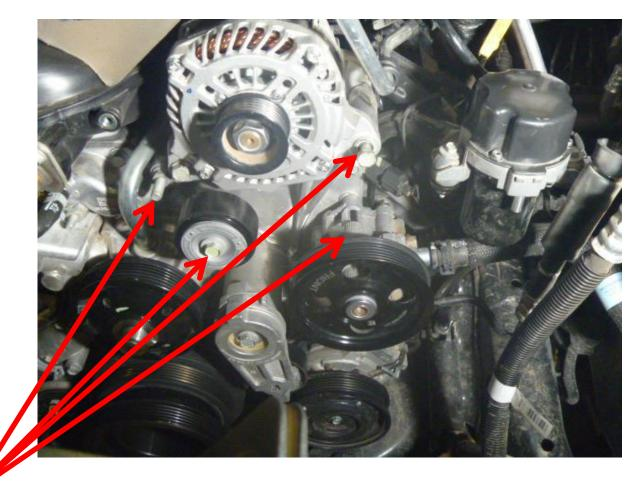
Remove the bolts from these locations. Remove the standoff for the air conditioner lines.
