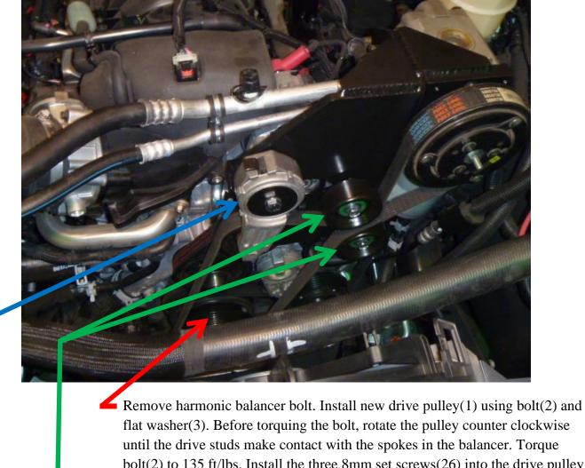
until the drive studs make contact with the spokes in the balancer. Torque bolt(2) to 135 ft/lbs. Install the three 8mm set screws(26) into the drive pulley from the inside. Run them all out until they touch the damper evenly. Then, tighten each set a little at a time until you reach 15-20 inch pounds.
