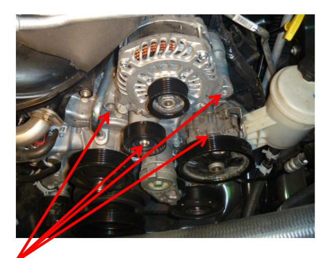
Remove the bolts from these locations. Remove the standoff for the air conditioner lines.
