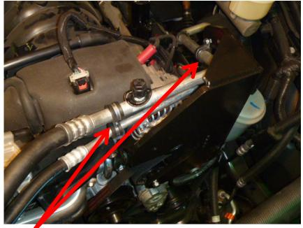
Install clamps(19,20) using bolts(21), lock washers(22) and nut(23).
