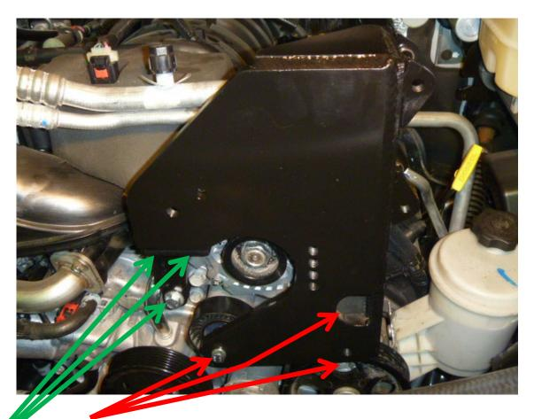
Install main bracket(5) using bolts(7,8,9) and lock washers(10,11).
