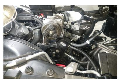
Kit Assembly (As Shown: Auxiliary A/C Compressor)
