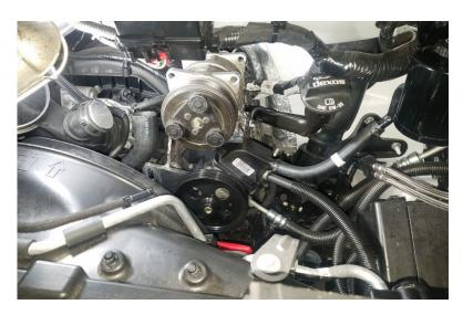
Kit Assembly (As Shown: Auxiliary A/C Compressor)
