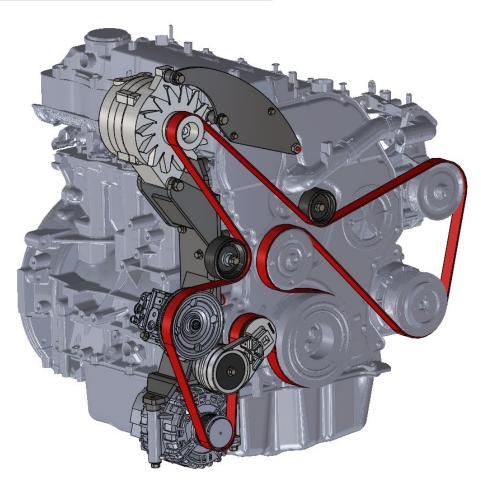
Install belt(25) according to the diagram above (belt will run on the back-seven grooves of the alternator). Readjust idler if necessary. Check belt alignment.
