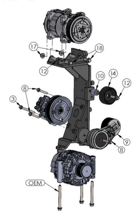
Install the auxiliary A.C. compressor using hardware (12,16,17,18). Install tensioner (9) using bolt (8). Install idler (14) with short bushing (10) and bolt (12) onto the bracket into one of the three tapped holes. The idler will usually need to go in the top hole. Replace the 2 ½ stamped steel OEM idler that is located just below the upper radiator hose with the 2 ½ machined steel idler (14) using long bushing (13) and bolt (15).
