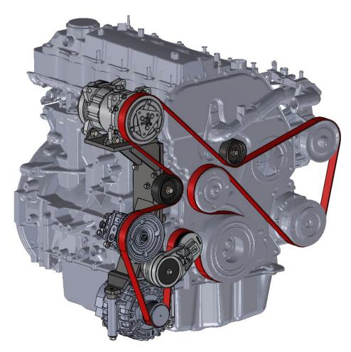
Install belt(19) according to the diagram above (belt will run on the back-seven grooves of the compressor). Readjust idler if necessary. Check belt alignment.
