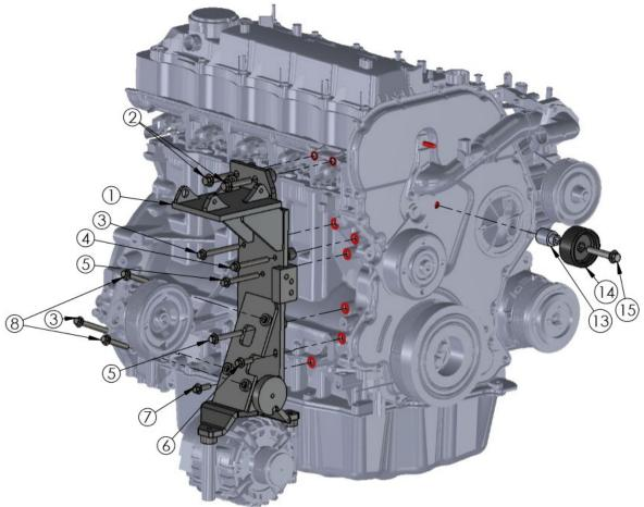
Install new bracket(1) as shown above using bolts(2-7). Install the alternator onto the bottom of the bracket reusing the O.E.M. bolts. Install the power steering pump onto the bracket using bolts(3,8).
