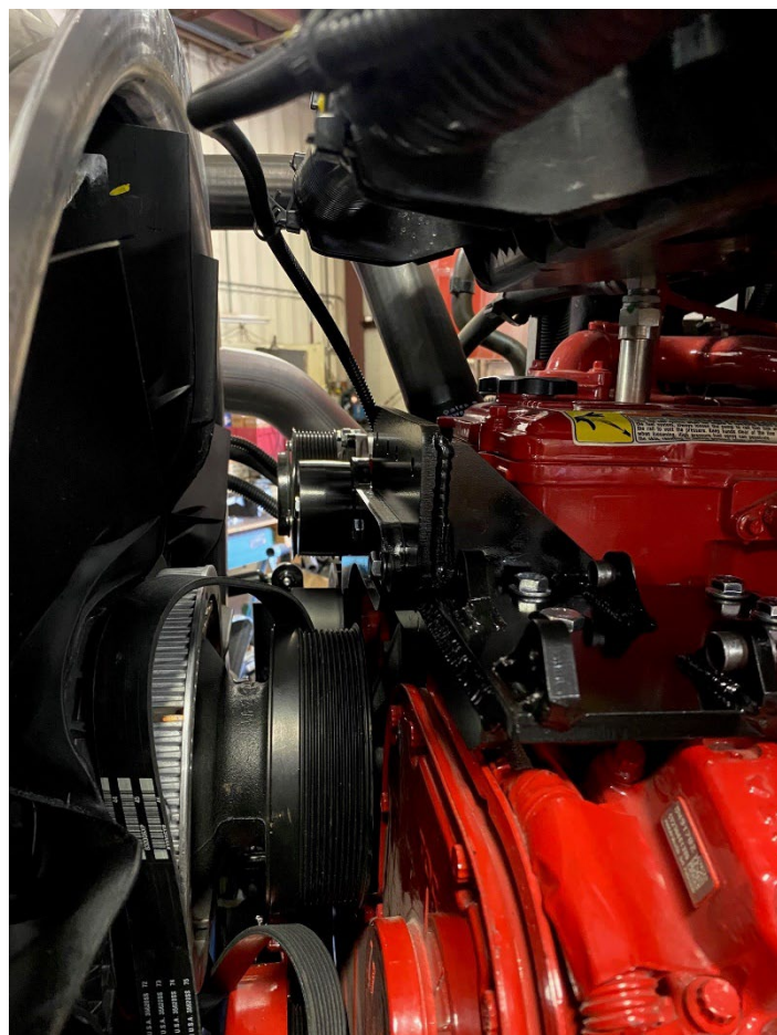
Main Bracket Installed (As Shown for Auxiliary A/C Compressor Application)
