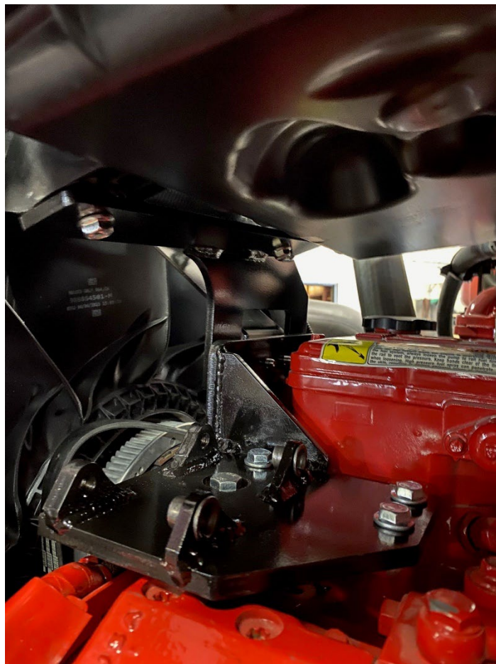
Air Cleaner Support Bracket Installed
