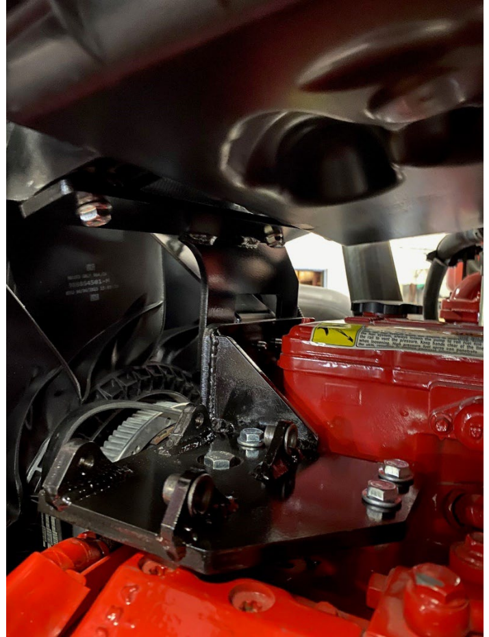
Air Cleaner Support Bracket Installed
