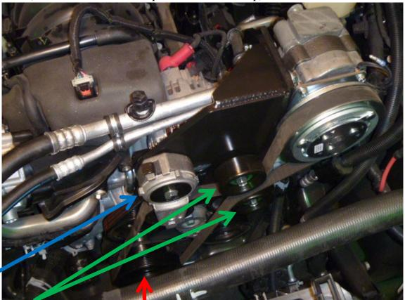
Remove harmonic balancer bolt. Install new drive pulley(1) using bolt(2) and flat washer(3). Before torquing the bolt, rotate the pulley counter clockwise until the drive studs make contact with the spokes in the balancer. Torque bolt(2) to 135 ft/lbs. Install set screws (4), installing finger tight then cross torquing by 20 in/lbs. increments to 100 in/lbs
