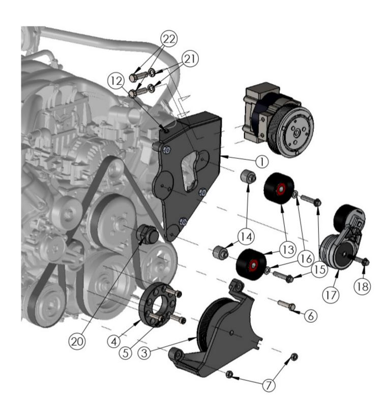
IMK534-8SB-5.5 2016-2019 Ford F650-750 6.8L V10 3 Valve W-WO AC W/Bearing Support
