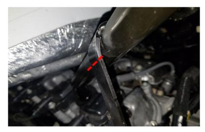
Oil Tube Bracket (Cut at Red Dotted Line)
