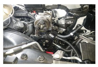
Kit Assembly (As Shown: Auxiliary A/C Compressor)
