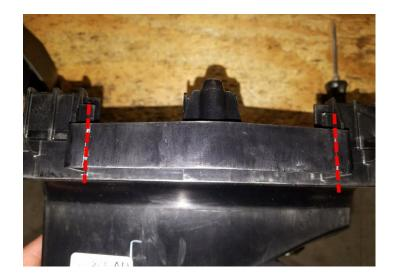
Air Cleaner Box Assembly (Cut at Red Lines)
